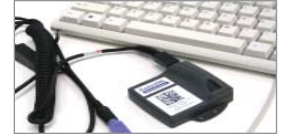
PS/2 Cable installed to CodeXML Modem & Keyboard
